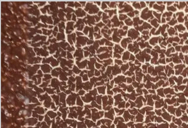
Photo 1: This photo shows mud cracking, which may be caused by a variety of issues related to stress.
