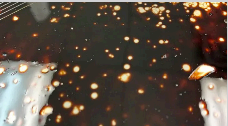
Photo 2: This photo shows cissing and dimpling, also known as fish eyes. This is caused by surface defects.
