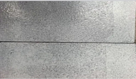
Photo 3: This photo shows grinning; another potential roof coating system failure.
