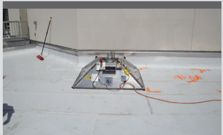
Negative pressure test or “bubble test.”
